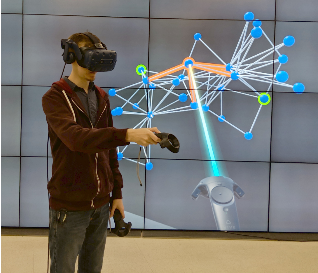
Figure 1.1. A user interacts with a 3D graph with the HTV Vive Pro HMD and controllers. The display mirrors the user's view. We compare this method of graph visualization with traditional desktop 2D graph visualization to determine how it effects users' mental maps.
